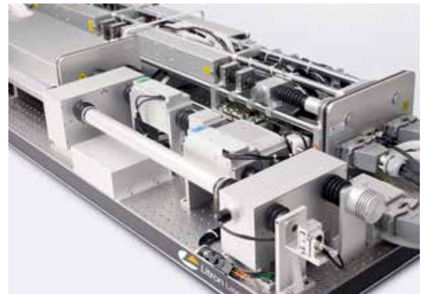
LPY10J laser system showing 2nd and 3rd harmonic stages.
